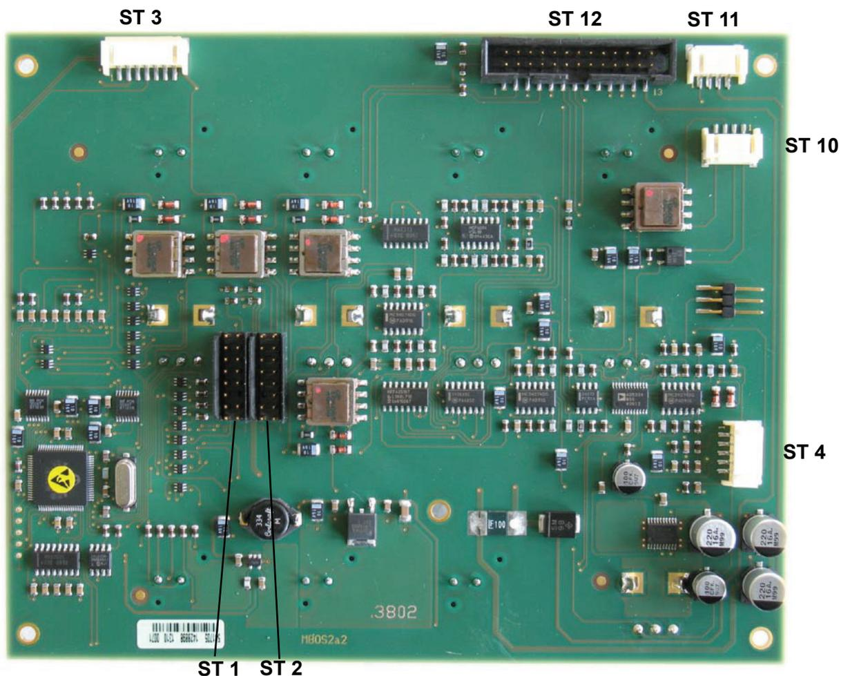
**Socket ST1, ST2, ST10, ST12 --> Connection Board**
